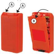
Position six alkaline batteries as indicated by polarity markings on inside of battery holder housing.
